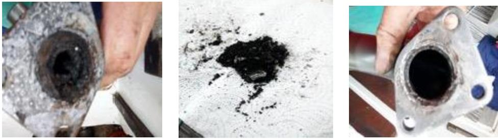
While this was maybe the cause it was not the problem. So, the cylinder head had to come off. Which revealed a broken exhaust piston. I bought a new piston cleaned the head up and ground in both pistons. You can see the amount of carbon I got out of the exhaust chamber in the cylinder head.
